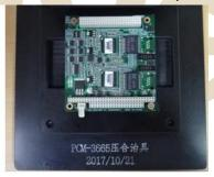
2. Put your board on PCM SBC board and align the two connectors, and then press the red handle of fixture.
